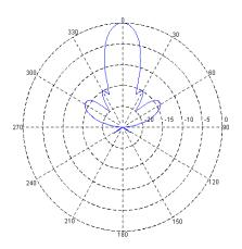
E-field radiation pattern (azimuth for horizontally polarized antenna)
