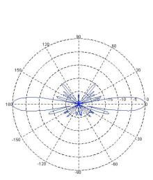
Elevation (E-field) radiation pattern
